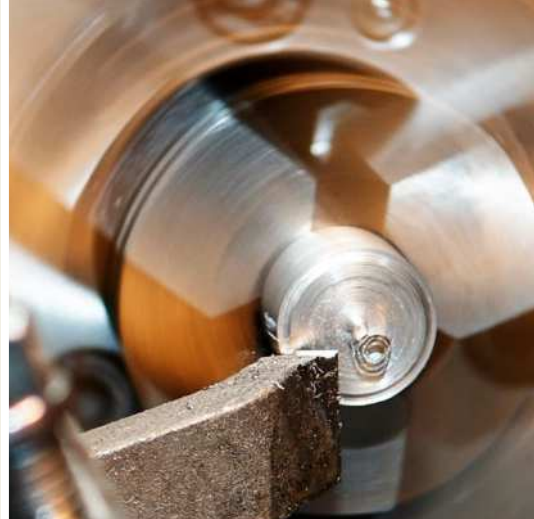
Counterbores for solderless tube connection (DIN 3854/DIN 3862)
