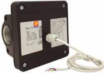
Art. 092-5170-110 Mechanical pulsed flow meter MGI-110 min-max flow rate 5-110 l/min nr. 41 pulses/liter
