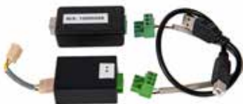
Art. 092-5350-001 Codified Kit Lan Connection USB-RS485
